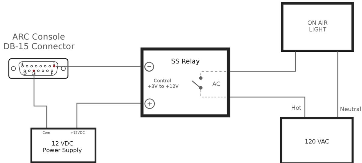
Due to the variety of products that are available we do not have a specific unit that we would recommend. However the key issue is to isolate the audio console from the on air lights AC voltage and still provide the necessary on off control. The circuit above should handle this interface issue with a minimum of wiring and components.
